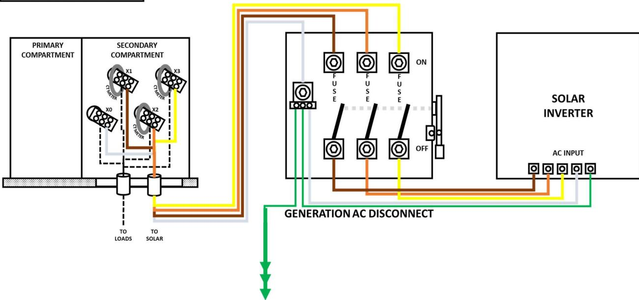
**POI: NEW WEATHERHEAD AT EXISTING SERVICE WITH EXISTING UTILITY METERING AT THE WEATHERHEAD (SOLAR AND/OR BATTERY)**
