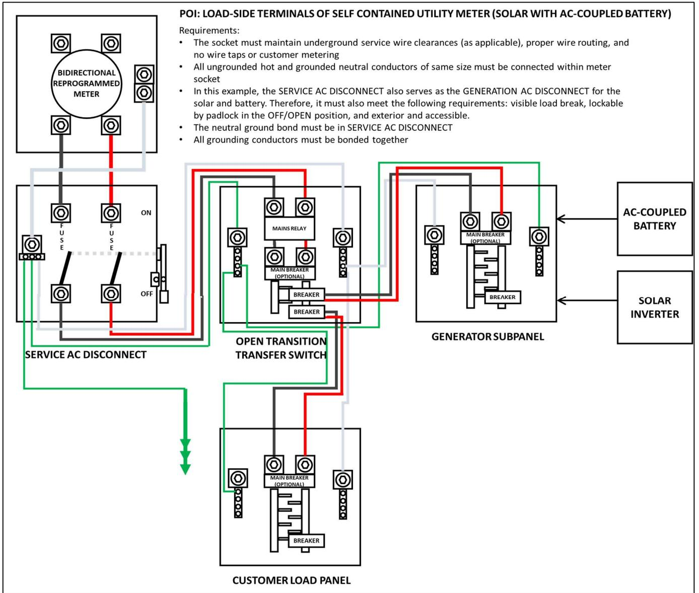
**POI: LOAD-SIDE TERMINALS OF SELF CONTAINED UTILITY METER (SOLAR WITH AC-COUPLED BATTERY)**
