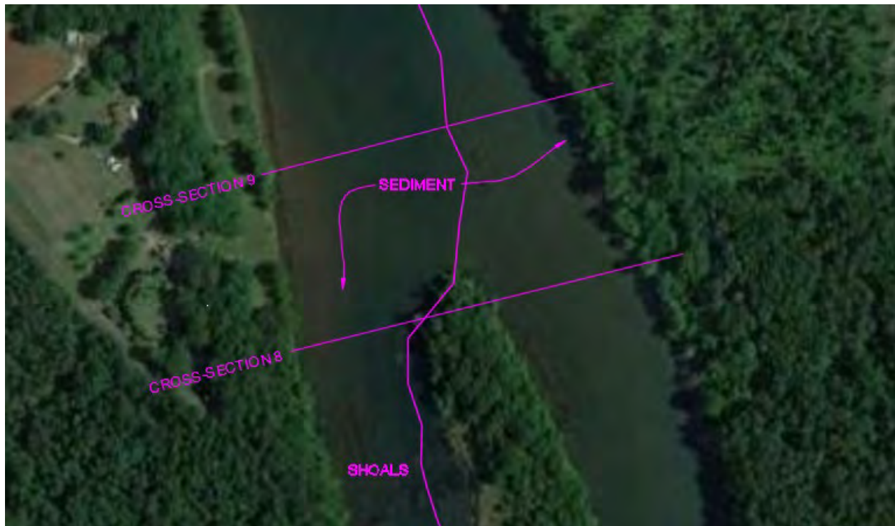
FIGURE D-4: SHOALS AND NATURALLY OCCURRING SEDIMENT NEAR CROSS SECTIONS 8 & 9 IN SECTION 4 (UPPER LANGDALE)
