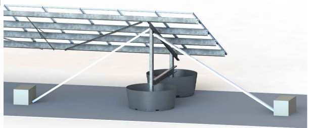
Temporary Bracing with Ballast Blocks
