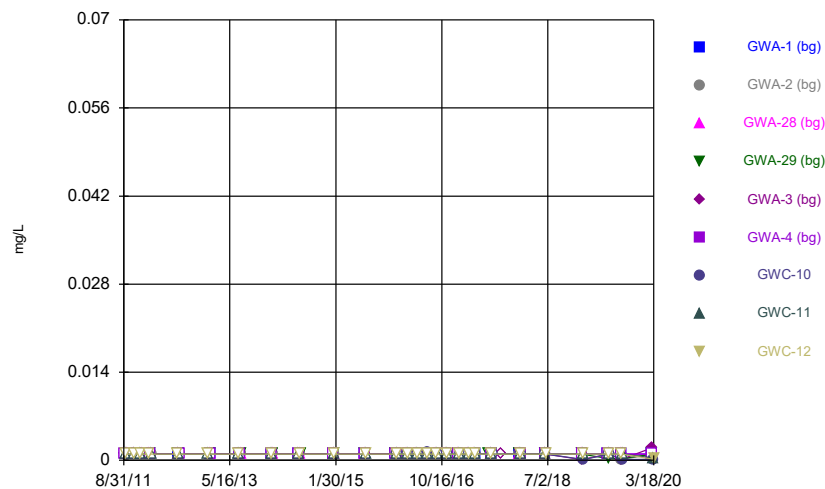
Constituent: Lead Analysis Run 5/20/2020 1:28 PM Plant Wansley Client: Southern Company Data: Wansley Landfill
