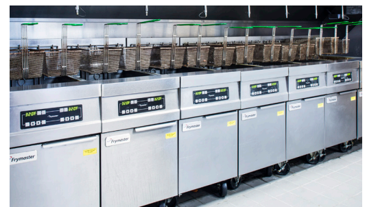
These new electric fryers not only use less energy, but they also reduce ambient heat in the kitchen.
