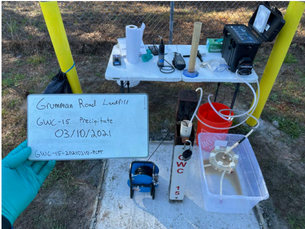
Photograph 1: Groundwater and precipitate sampling site setup showing a peristaltic pump and in-line filter stand
