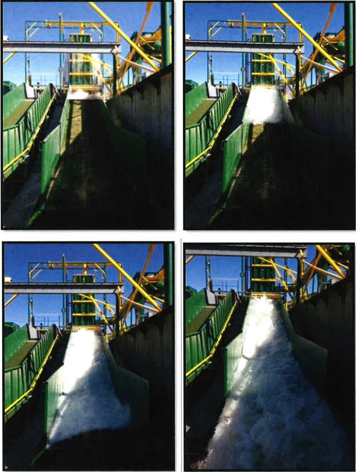
Figure 26 – Wave Overtopping Testing of HydroTurf® at CSU
