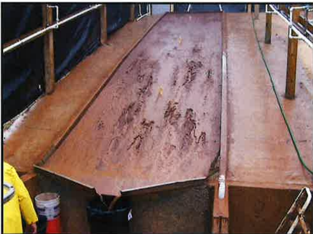
Typical Unprotected Slope Erosion from Testing Protocol (2 in/hr on left; 6 in/hr on right)
