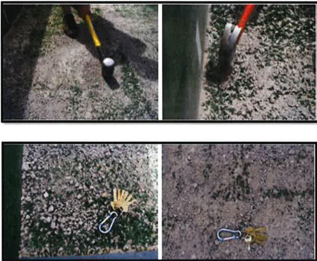
Figure 23 – Intentional Damage: Pulverization of HydroBinder® Infill
