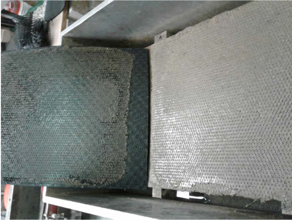
Figure 5. MicroDrain (Microspike side) and subgrade soil surfaces at the completion of test #1D at 75 psf.
