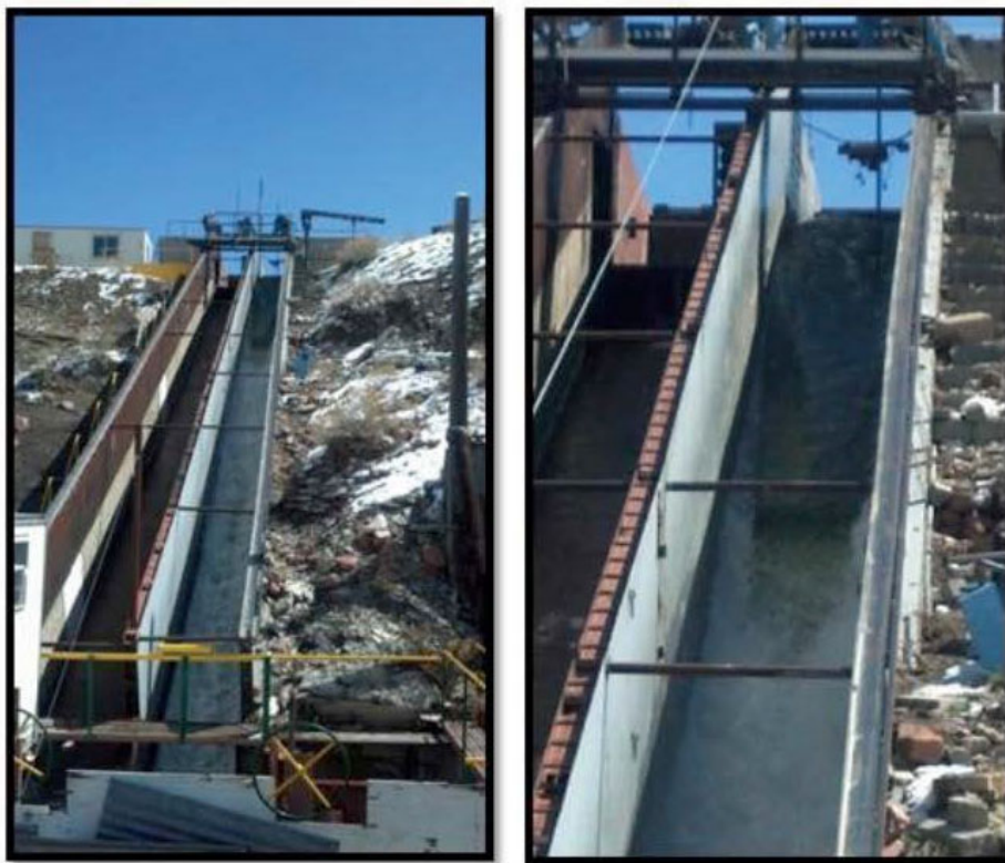
Figure 6.5 – Steady State Hydraulic Testing of HydroTurf™ at CSU
