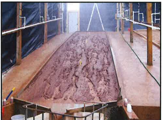
Typical Unprotected Slope Erosion from Testing Protocol (2 in/hr on left; 6 in/hr on right)
