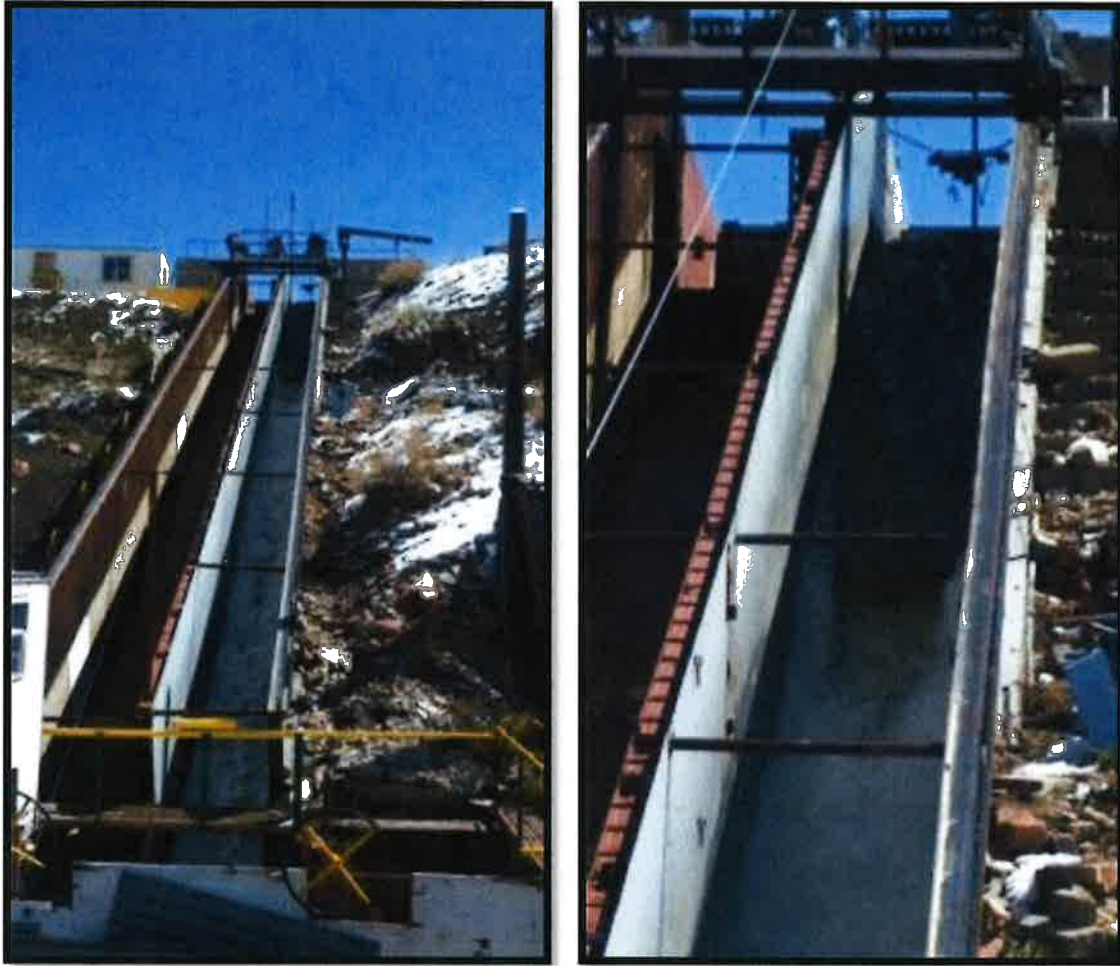
Figure 6 – Steady State Hydraulic Testing of HydroTurf® at CSU
