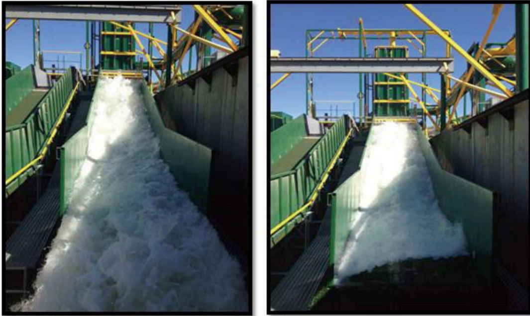
Figure 6.6 – Wave Overtop Hydraulic Testing of HydroTurf® at CSU
