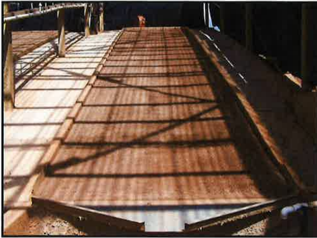
Test Slope Prepared and Liner Installed
