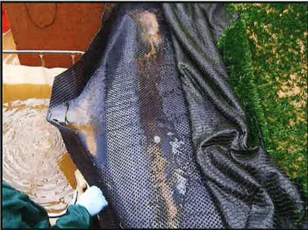
Only Small Amounts of Sand Migrated Within the Drainage Layer and Little Sand Movement Was Observed On Surface
