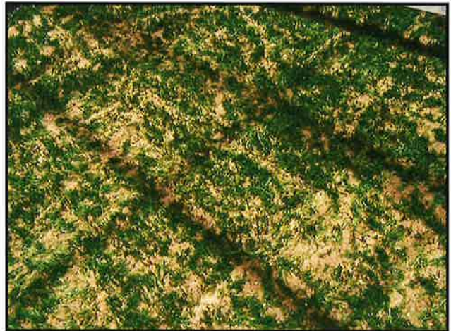
Only Small Amounts of Sand Migrated Within the Drainage Layer and Little Sand Movement Was Observed On Surface
