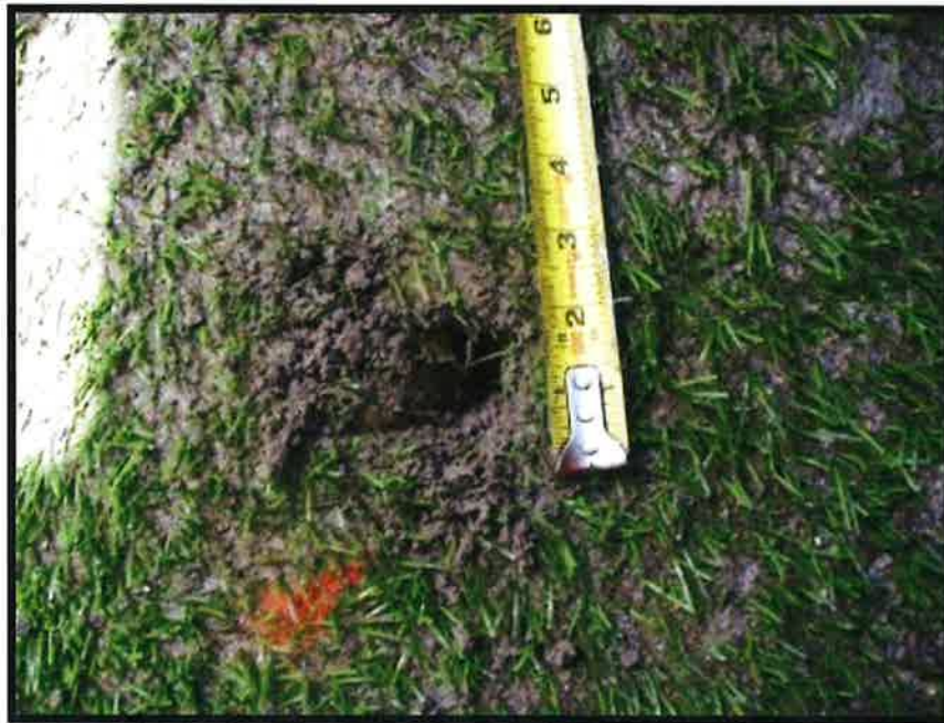
Figure 17 - Intentional Damage: Hole from Pick Ax (Prior to Testing)
