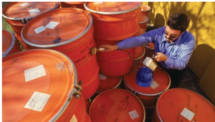
Health physics technician surveying barrels for radiological contamination
