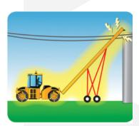
Lower a portable grain auger before moving.
