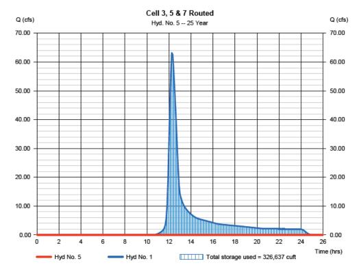
Cell 3 shows an outflow of 0.00 cfs because the Peak Water Surface Elevation of 688.73 is lower than the top elevation of the riser structure which is 690.10. However, the riser structure is perforated to allow flow out of the sedimentation and clear pool. That flow is not modeled due to its very minimum.
