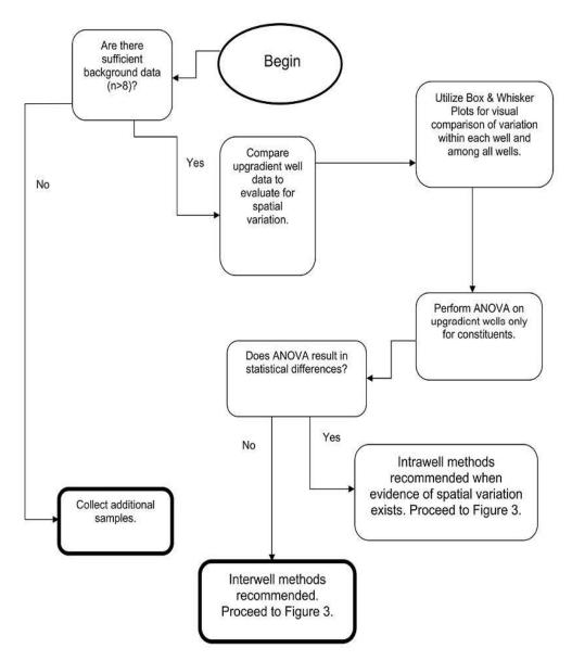
Figure 3: DECISION LOGIC FOR COMPUTING PREDICTION LIMITS
