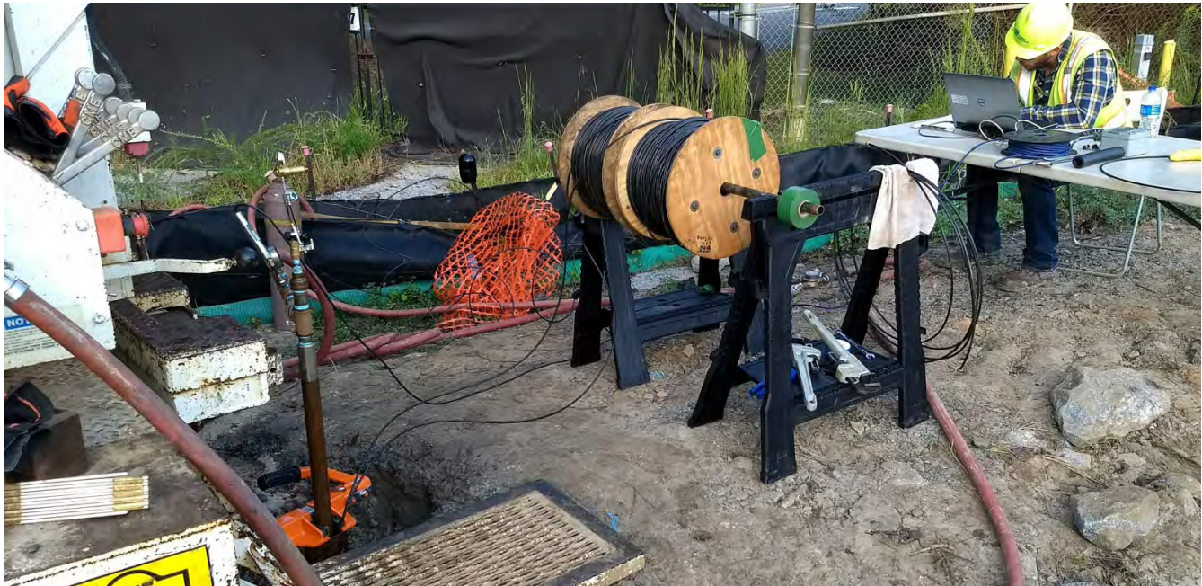
Figure 3.3: Photo of Hydrogeological Testing Setup at Surface
