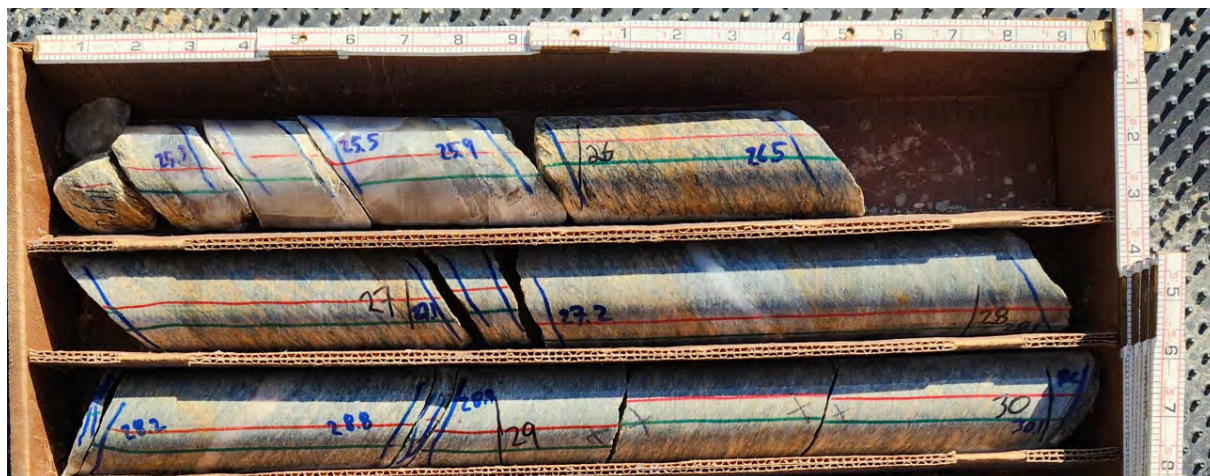
Figure 2.1: Rock Core Photo showing the Long Island Creek Gneiss formation from BW-5, 25 to 30 feet below Existing Ground Level
