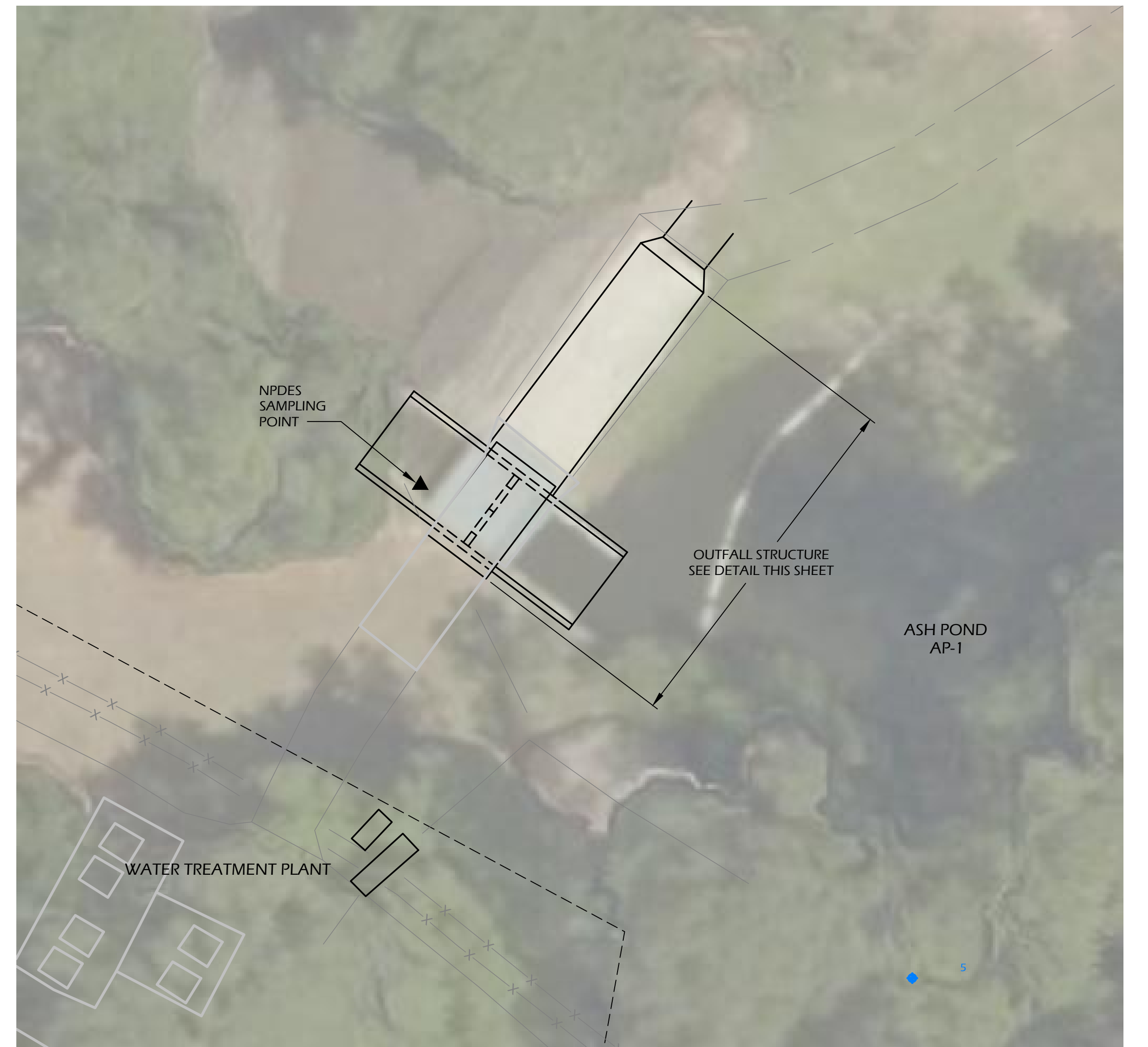
EXISTING NPDES OUTFALL STRUCTURE AREA SCALE: 1" = 10'
