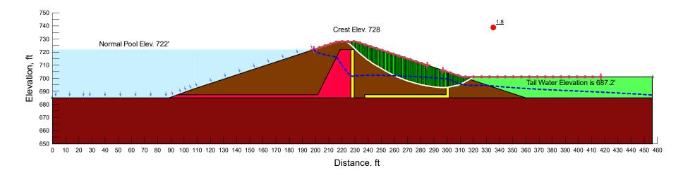
Loading Condition: Steady State Seepage with Normal Pool Condition (Effective Strength Parameters)
