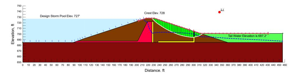
Loading Condition: Steady State Seepage with Design Storm Pool Condition (Effective Strength Parameters)
