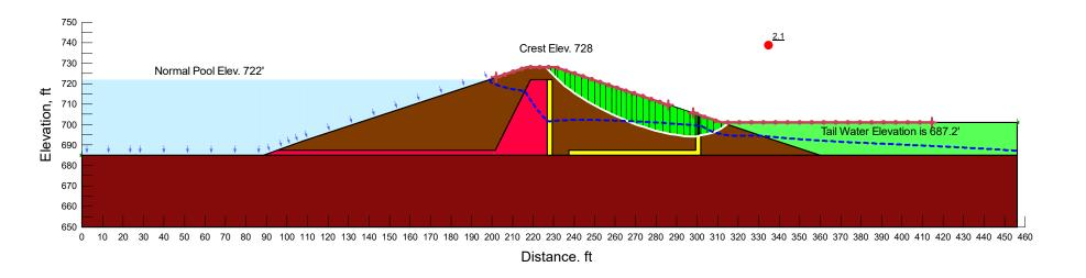
Loading Condition: Steady State Seepage with Normal Pool Condition (Effective Strength Parameters)
