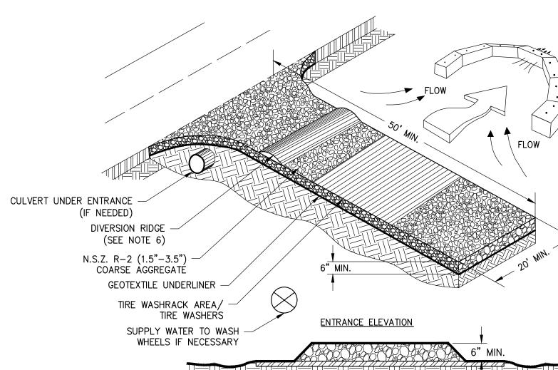
. AVOID LOCATING ON STEEP SLOPES OR AT CURVES ON PUBLIC ROADS. 2. REMOVE ALL VEGETATION AND OTHER UNSUITABLE MATERIAL FROM THE FOUNDATION AREA, GRADE, AND CROWN FOR POSITIVE
