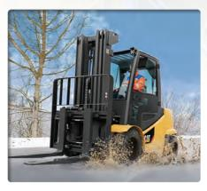
whether Class 1 electric or Class 5 IC, have pneumatic tires to improve handling on rough surfaces. They also have enclosed motors and electronic systems to ensure safe operation in wet, dusty, windy conditions, and sometimes have an enclosed cab for the driver.
