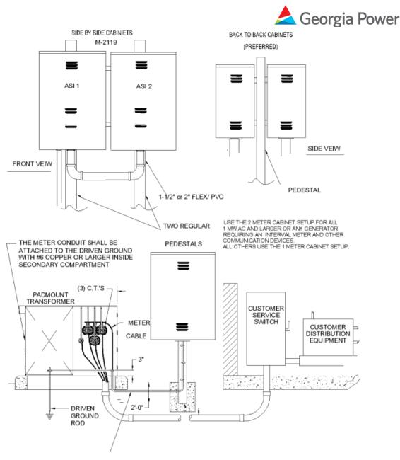
1-1/2" SCHEDULE 40 PVC, TRADE SIZE THREADED RIGID OR INTERMEDIATE METAL CONDUIT FURNISHED AND INSTALLED BY CUSTOMER.
