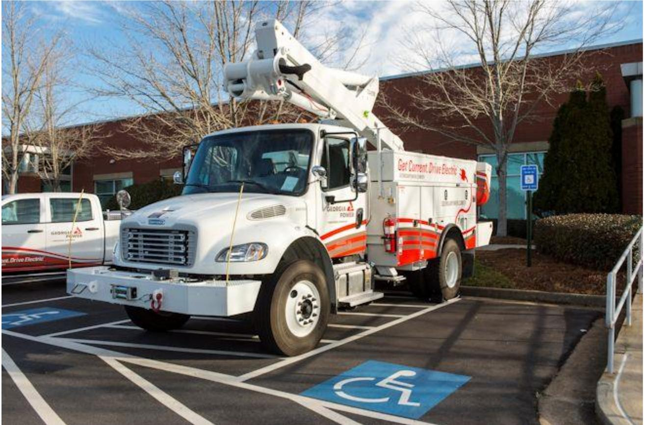
As the name implies, the hybrid bucket truck operates with both a biodiesel internal combustion engine and an electric motor. The biodiesel engine operates while driving on the road, but when it comes to bucket work, the electric motor takes on the main role.
